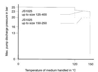
The diagram refers to the components under pressure, i.e. the pump casing and discharge cover.
